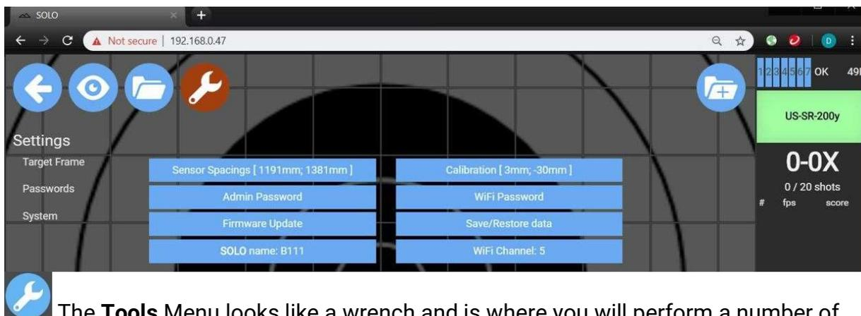
The **Tools** Menu looks like a wrench and is where you will perform a number of maintenance functions such as frame sensor spacing, calibration, optional passwords, update firmware, data maintenance, target name, and WIFI channel.
